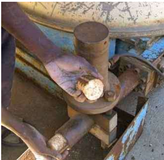
Briquette-making from saw-dust with a hydraulic press in Karamoja (Uganda)
