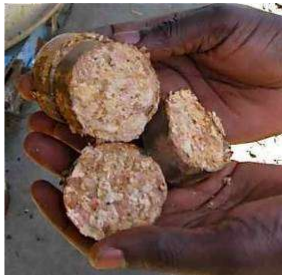
Briquette-making from saw-dust with a hydraulic press in Karamoja (Uganda)
