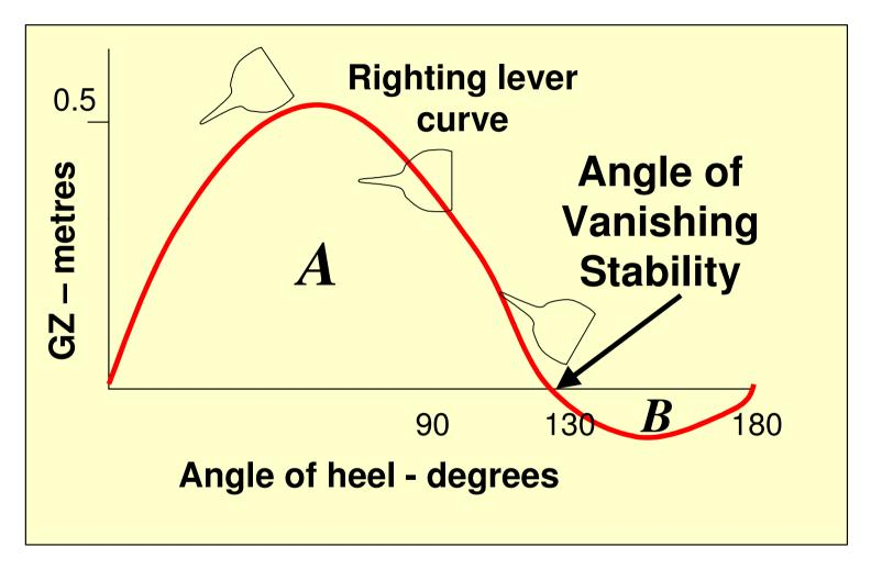
Area 'A' indicates the resistance of boat to capsize Area 'B' indicates wave energy required to right the boat
