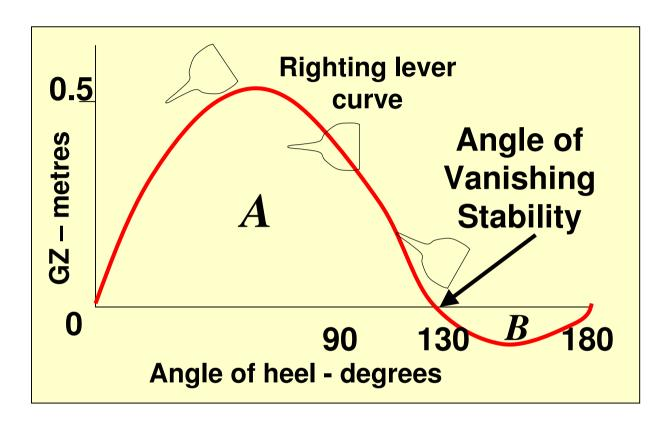
Area 'A' indicates resistance of boat to capsize Area 'B' indicates wave energy required to right the boat
