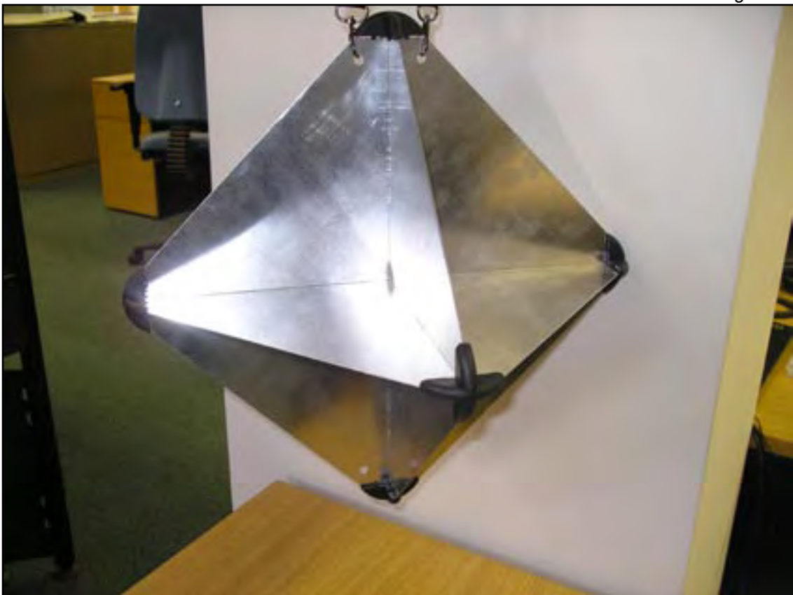
Radar reflector (not in "catch rain" position) suspended from the fixing points
