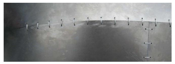
Wire connection works better than staples – stronger pull. It is more flexible and gives better pulling control. But staples prevents seams from "overriding" and keep metal edge-to-edge.
