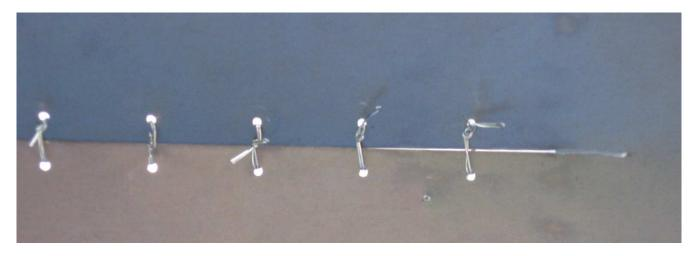
For stitching second half of the pattern I used 24ga galvanized steel wire from Home Depot. I made 2 strands from it and secure it by twisting together. It made pretty strong connection.
