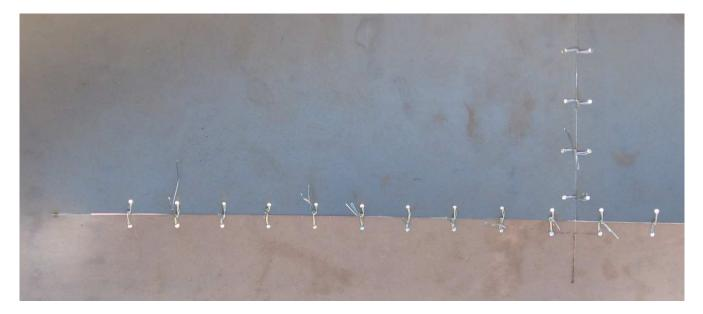
You can see some gap at the end of the dart. This is because it was need to open the dart's end a little bit more. My "scoring" allowed to fold pattern easier, but it did not cut metal deep enough to go all the way through and make the dart narrower. There is almost NO GAP between the seams of the pattern edge to edge along the seam away from the end of the dart.
