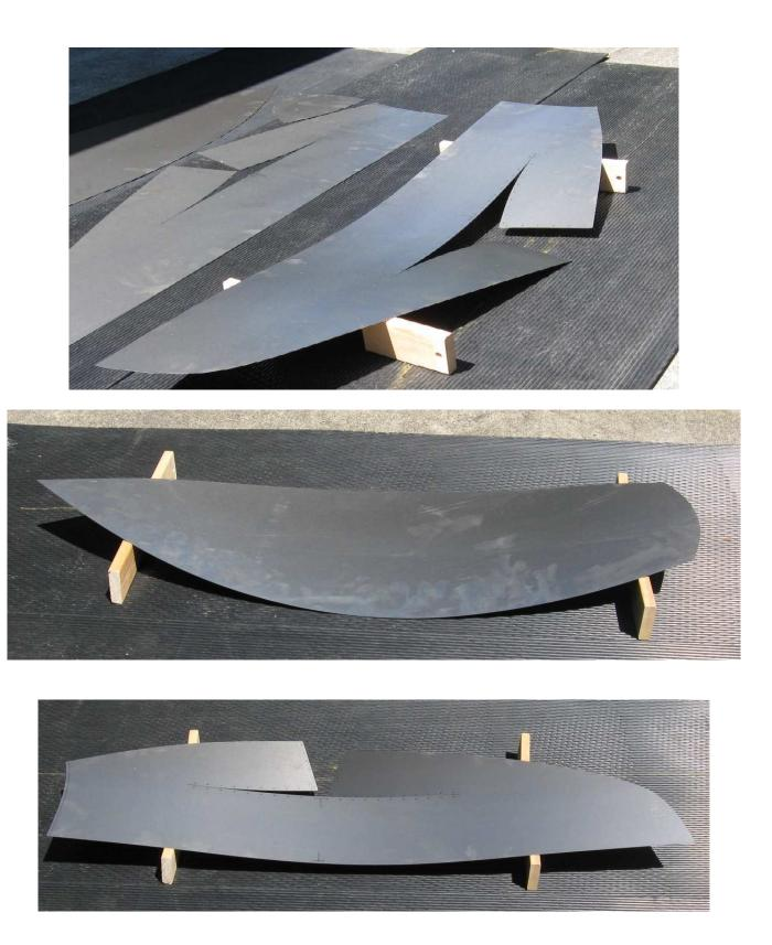
As you can see, flat 24ga steel sheet is pretty floppy. Origami hull will gain it strength step by step. Following Brent's recommendations and sequence for folding the hull you should not have any problems to get strong and perfectly fit hull.
