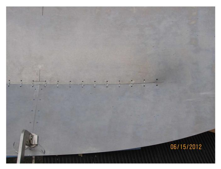
I found that making lower midships seam flat when you fold the hull, make the seams edges much easier to fit correctly. It could be done by welding temporary straight edge (or angle) to the pattern before pulling pattern together.
