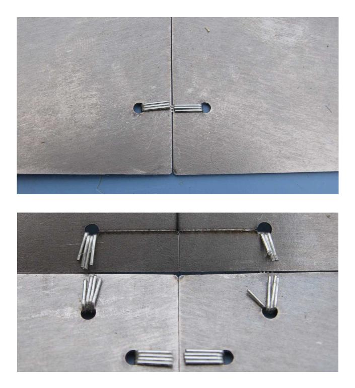
You can see some gap at the join of the seams. This is because it is hard to bend several staples and keep uniform tension. Another problem is that the ends of staples are not connected and the links expand slightly under the force of pre-tensioned metal. The joints are exactly where it suppose to be. Small gaps will be eliminated with better holding media.
