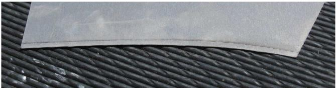
Because of limitation of laser-cutting equipment, it was impossible to cut the dart as far as necessary. I had to find a compromise. Uncut portion of the dart was just marked (engraved) by laser for reference (top picture). It gave me an idea to mark midships marks (middle picture) and extend the hull for easier fitting of the transom. Original position where the transom suppose to be was engraved on hull's pattern (bottom picture).
