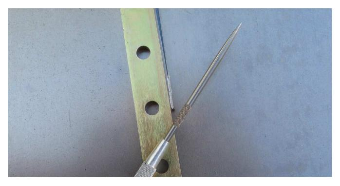
This tool worked MUCH better. I was able to make deeper and narrower groove in 24ga metal than using "micro grinder". It took some elbow grease to do it, but modeling is serious business ;))
